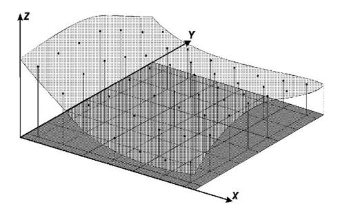
The rectangle grid generation must be done when a sampled data in the surface is not obtained with regular spacing. Thus from isoline contained information or in sampled points it is generated a grid that represent as closest as possible to the real surface. Initial values to be determined are x and y coordinate space in a way they can represent close values to the grid points in big variation regions. At same time, they should reduce redundancies in almost plane regions.
