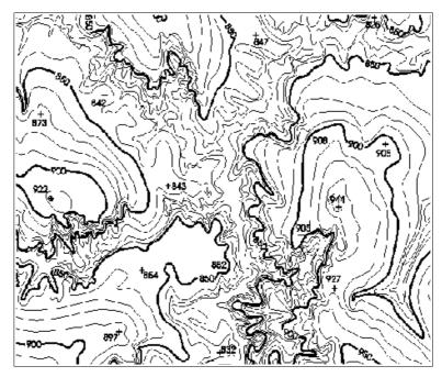
Isolines can be viewed like a plane projection (x,y) of intersections between the surface and equidistant horizontal planes.
