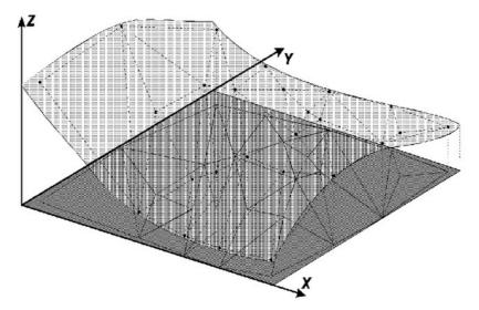
The redundancy number is drastically reduced if compared to the rectangle grid, once the grid is thinner in regions of big variations and more spaced in almost plane regions. Surface discontinuities can be modeled through characteristic lines and points.
